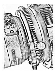
Now slip the iris scale to line up the lens f- number with the index line on the adapter.
